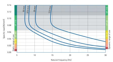
Natural frequency of a single-degree-offreedom system consisting of a fixed mass and an elastic bearing consisting of VIKAFOAM VF 65 on a stiff subgrade.
